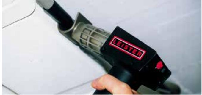
Shrinking cable connections with the GHIBLI.
