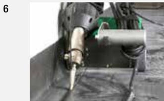
The 51 mm/2 inches minimum distance from the wall, ensures trouble-free welding around construction pipes and L-skirts. Due to its compact height, the MINIFLOOR seamlessly welds beneath obstacles with a minimum clearance of 295 mm /12 inches.
